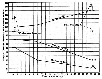
Frg. 100.—Theoretical conditions in kiln while drying lumber 2 inches thick of the lighter pines, spruces, etc.
